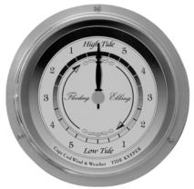
side of the dial, the tide is rising and the numbers indicate the number of hours before high tide; when the hand is on the right side of the dial, the tide is falling and the numbers indicate the number of hours before low tide.
